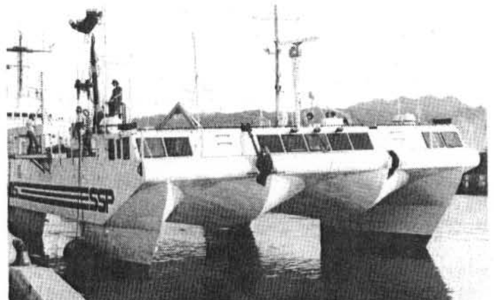
The SSP KAIMALINO is a Navy-owned SWATH vessel (small waterplane area twin hull); its design is being considered for future oceanographic research vessels. Photo by Bob Dinsmore.
