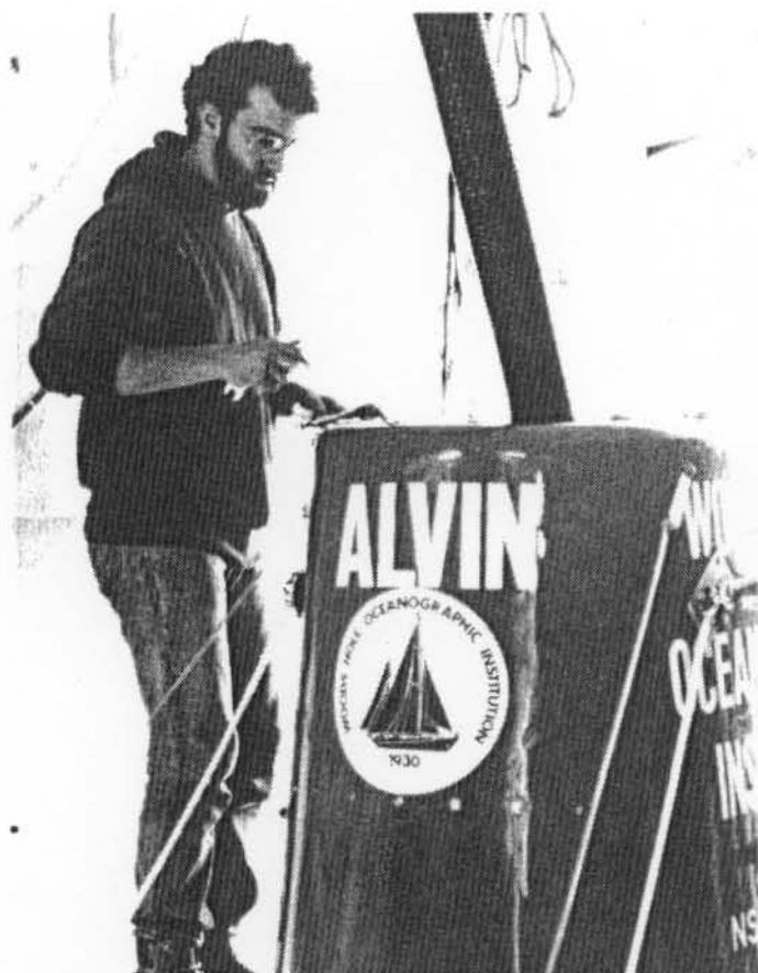
Jim Hardiman bleeds sail lines during routine ALVIN maintenance procedures.
