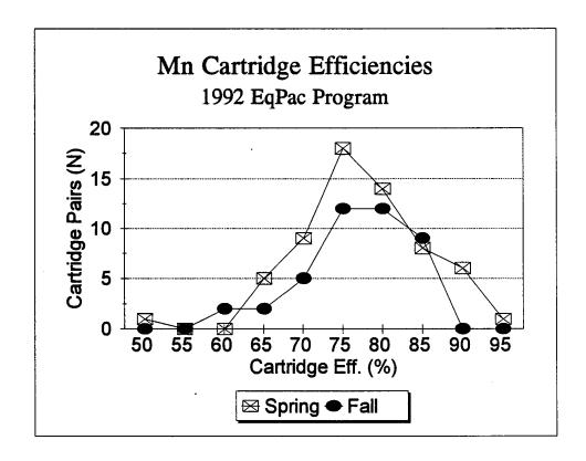
The collection efficiencies for the spring and fall legs plot into a typical Gaussian distribution, with the highest number of cartridge pairs falling at or near the mean collection efficiency of 0.79 + /-9% (percent cartridge efficiencies are rounded to the nearest 5%). This mean collection efficiency is consistent with that of the 10-inch Micro-wynd II, previously used by this laboratory (0.87 + /-8%, n = 40; Buesseler et al., 1992b).
