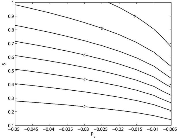
FIG. 3. Interior alongshelf velocity  $u^i$  from the theoretical model after 10 friction time scales, relative to the unstratified steady-state velocity, contoured over a range of downwelling pressure gradients and Burger numbers.
