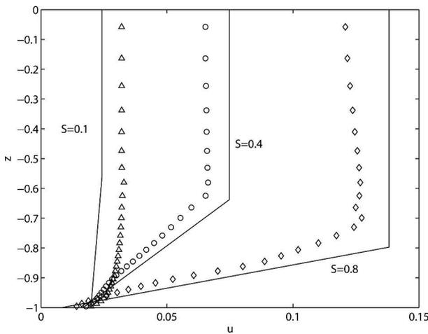
FIG. 7. Comparison of the theoretical (solid curves) and numerical model (symbols) velocity profiles at  $t = 8$  and  $y = 70$  km offshore in response to a downwelling pressure gradient of  $P_x = -0.02$  and for several Burger numbers. All variables are scaled as stated in text.
