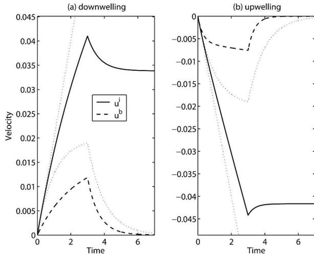
FIG. 12. Theoretical interior and bottom velocities in response to forcing of finite duration. A (a) downwelling or (b) upwelling pressure gradient is imposed until  $t = 3$  and is then removed, with  $S = 0.4$  and  $P_x = \pm 0.02$  (and  $r/fh = 0.0625$  for upwelling). Dotted straight lines show the response with no bottom friction. Dotted curves show the response with no stratification ( $S = 0$ ).
