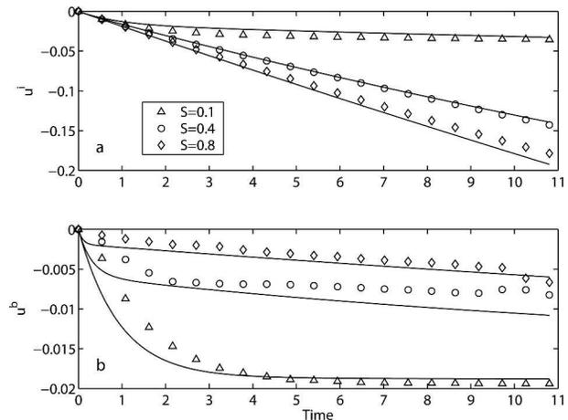
FIG. 10. Comparison of the theoretical (solid curves) and numerical model (symbols) time responses to an upwelling pressure gradient of  $P_x = 0.02$  and for several Burger numbers ( $S = 0.1, 0.4, 0.8$ ): (a) interior and (b) bottom velocities at  $y = 70$  km offshore. All variables are scaled as stated in text.
