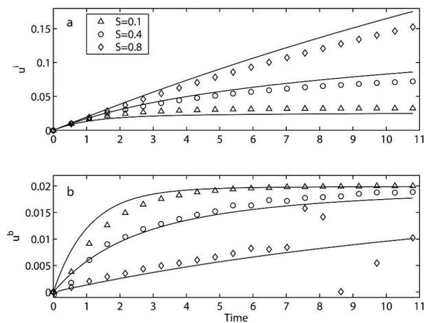
FIG. 6. Comparison of the theoretical (solid curves) and numerical model (symbols) time responses to a downwelling pressure gradient of  $P_x = -0.02$  and for several Burger numbers ( $S = 0.1, 0.4, 0.8$ ): (a) interior and (b) bottom velocities at  $y = 70$  km offshore. All variables are scaled as stated in text.
