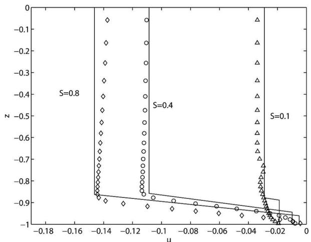
FIG. 11. Comparison of the theoretical (solid curves) and numerical model (symbols) velocity profiles at  $t = 8$  and  $y = 70$  km offshore in response to an upwelling pressure gradient of  $P_x = 0.02$  and for several Burger numbers. All variables are scaled as stated in text.
