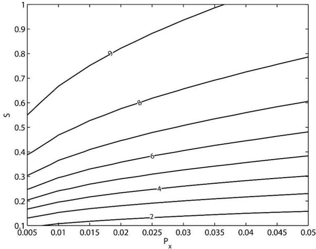
FIG. 5. Interior alongshelf velocity  $u^i$  from the theoretical model after 10 friction time scales, relative to the unstratified steady-state velocity, contoured over a range of upwelling pressure gradients and Burger numbers ( $r/fh = 0.0625$ ).
