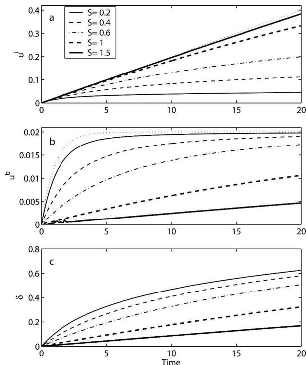
FIG. 2. Response to a downwelling pressure gradient ( $P_x = -0.02$ ) for various values of Burger number  $S$ : (a) interior velocity, (b) bottom velocity, and (c) bottom boundary layer thickness. All variables have been scaled as stated in text. Dotted line in (a) is the response with no bottom friction. Dotted curve in (b) is the response with no stratification ( $S = 0$ ).
