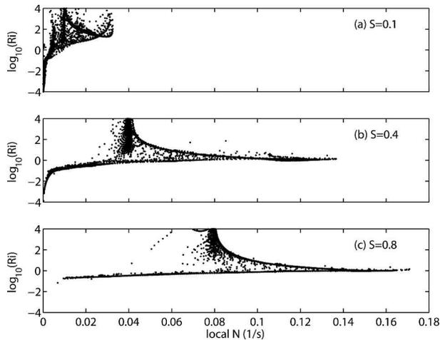
FIG. 9. Local gradient Richardson number at each grid point in the numerical model plotted against the local buoyancy frequency, for three different Burger numbers. The largest  $N$  occurs in the geostrophic shear layer, where  $Ri \approx 1$  for  $S = 0.4$  and  $0.8$ .
