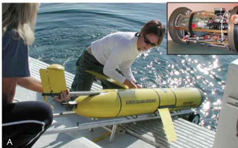
Figure 5. Optical detection of toxic Karenia species using BreveBuster . (A) Slocum glider fitted with optical instruments capable of detecting HAB species containing the unique carotenoid gyroxanthin-diester. The next three panels (B, C, D) show Karenia brevis similarity indices and remote-sensing data collected during a Slocum glider mission off the southwest coast of Florida from October 18–November 2, 2007. (B) A perspective plan view of the similarity indices; red symbols are locations where indices were over 0.6, the threshold value for presence of Karenia sp. (C) SeaWiFS chlorophyll satellite image from October 22, 2007. (D) An overlay of the other two panels. Note the collocation of red similarity indices and the chlorophyll filament extending southwest from the coast. Other red symbols that are not associated with the chlorophyll signal are still indicative of Karenia presence. In those cases, they were not of sufficient biomass to stand out as higher than background chlorophyll levels in the remote-sensing image.
