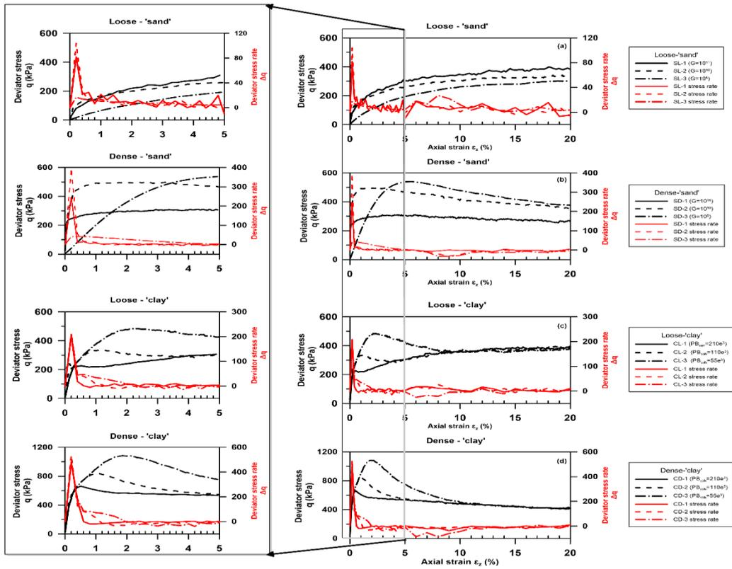
**Figure S2.** The stress rate was calculated for intervals of 1% of strain. The results are presented for samples tested under confining stress ( $\sigma_3=$ ) 250 kPa. Stress–strain curves are in black lines and stress rate in red lines. (a) loose 'sand' (b) dense 'sand' (c) loose 'clay' and (d) dense 'clay' samples. The rectangular inset in a-d represents zooming-in for the behavior between 0–5% of strain in the figures on the left for each material.
