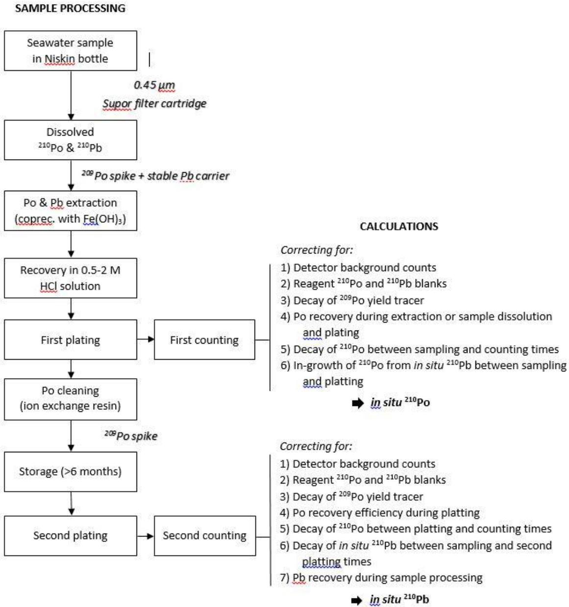
Figure 1: Flow chart of chemical processing for dissolved  $^{210}Po$  and  $^{210}Pb$ .
