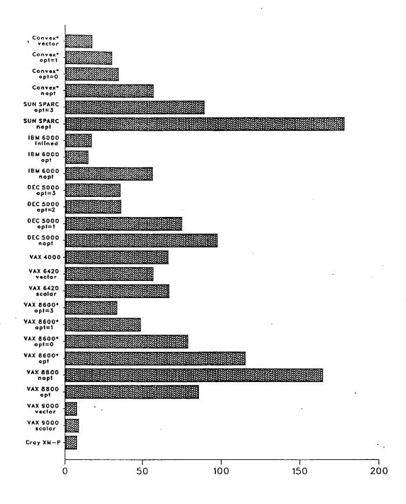
Figure 1: Comparison of benchmark times (in minutes) for the FINDIF code (\* denotes elapsed time; no star denotes CPU time)
