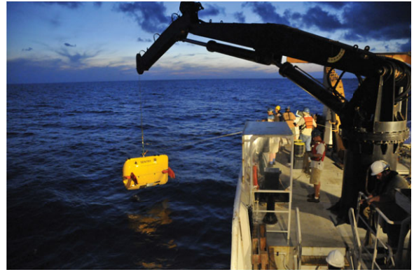
Figure 14. The National Deep Submergence Facility (NDSF) AUV Sentry is an unmanned oceanographic research vehicle that dives as deep as 6,000 m to perform various scientific missions. Sentry navigates primarily by DR with a FOG and DVL. The FOG is located in the main pressure housing, roughly amidship and just below the name label. The DVL is on the keel just aft from the bow. The large separation between these sensors on a vehicle that may deform under extreme pressure (even slightly) motivates our study of stable, in situ sensor alignment methods (photo credit: D Yoerger, ABE/ Sentry Group, WHOI).
