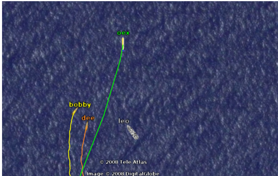
Figure A.4: GEOV screenshot showing ASCs Bobby and Dee trailing the OEX AUV to improve networking throughput at the CCLNET08 experiment. Acoustic communications are only robust over short distances with largely vertical propagation, which makes these “mobile gateways” effective, as they can always maintain a relatively short distance to the AUV. The ASCs were commanded to trail at 100 meters behind the AUV at 170° and 190° relative to the AUV’s bow. The ASCs were also running a high priority collision avoidance behavior with the RV Leonardo (“leo”), which accounts for the shift to port from the normative tracking positions.
