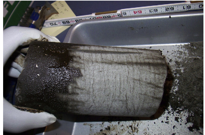
Fig. 3. Drilling mud being scraped away from a hydrate-bearing sandstone core recovered from the Mount Elbert well. Scale is in inches.
