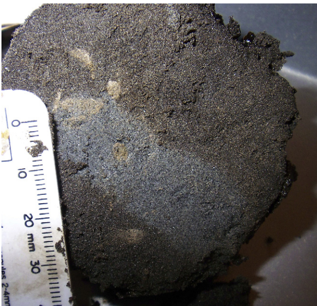
Fig. 2. Deep penetration of oil-based drilling mud into a coarse-grained sediment core recovered from the Mount Elbert well. Drilling mud penetrated deep into the core at several locations (Torres et al., 2011).
