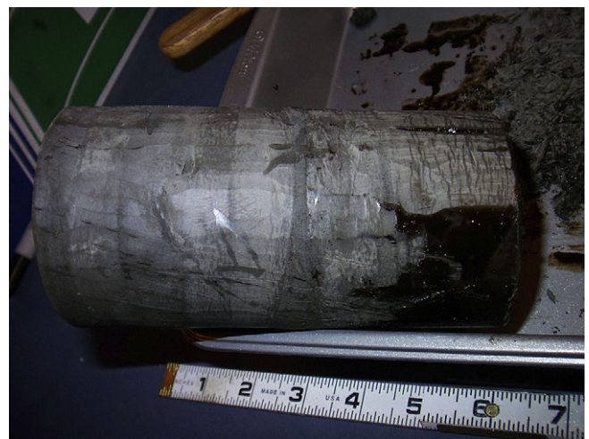
Fig. 4. Shale core recovered from the Mount Elbert well. Some coring disturbance is evident on the far right of the core. Scale is in inches, the industry standard unit of measure used in the field.
