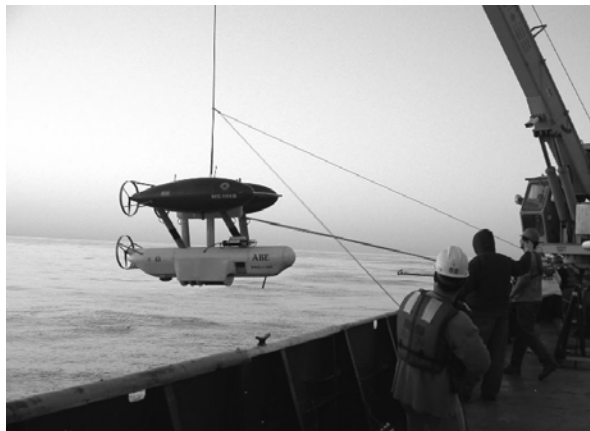
Fig. 2 Deployment of the Autonomous Benthic Explorer (ABE) vehicle.
