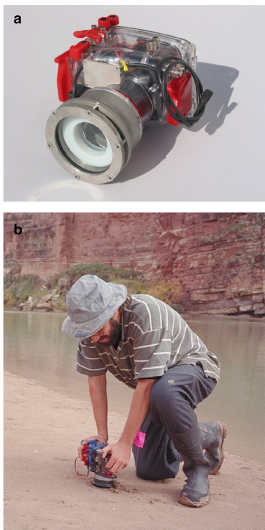
Fig. 3. Lightweight underwater microscope for hand-held use on beaches or by divers in shallow water. (a) Closeup of camera and housing; design follows requirements specified in Fig. 1. (b) Camera in use.
