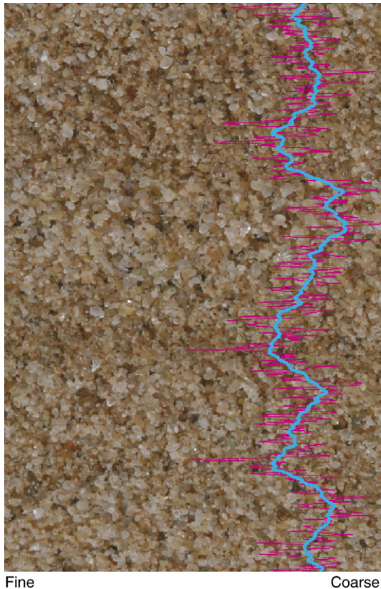
Fig. 7. Vertical profile of grain size through laminae deposited by wind ripples. Each wind ripple deposited a layer that coarsens upward (Hunter, 1977), followed by abrupt fining.
