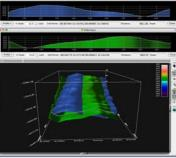
Fledermaus enables rapid detection of sound velocity and roll-bias problems in multibeam data.
