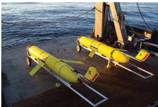
Fig. 1. Two Slocum gliders in summer 2003. Each is about 1.5 m long. Motion in the vertical plane follows a sawtooth trajectory. A rudder is used to steer in the horizontal plane. Maximum depth is 200 m and average forward speed relative to the flow is approximately 35 cm/s. During the AOSN 2003 experiment, the gliders were configured to surface and communicate as frequently as every 2 h.
