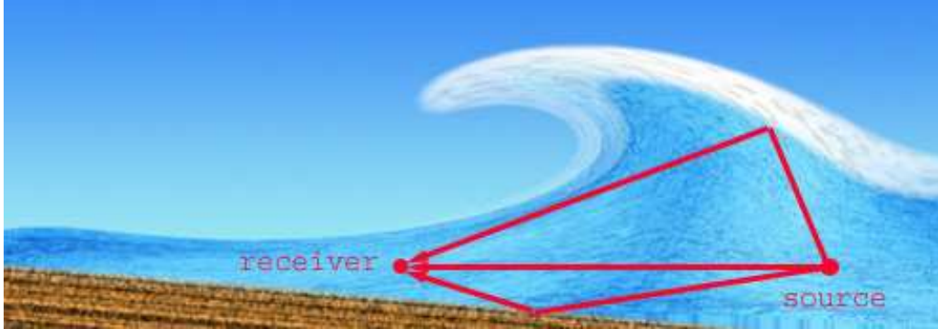
Figure 1-1: Acoustic Communications in Surf-Zone Channel. Surface waves are the dominant factor causing channel dynamics.
