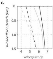
Figure S4. Tomographic models for Lines 9a and 9b. High velocities occur in the Central Dome and lower velocities are determined in the upper ~1.5 km on the southern dome. Dark-shaded areas have no ray coverage. a) Line 9b. b) Line 9a; location of IODP drill hole is indicated. c) Velocity-depth profiles at two similar locations along Line 9b (gray) and Line 9a (black), which is to the east (Figure 1). Dashed- Southern Ridge (arrow, -3.5 km); solid- Central Dome (arrow, +3.0 km).
