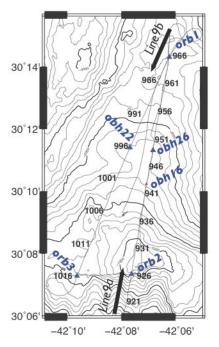
Figure S1. Details of the OBS refraction experiment at Atlantis Massif. Bathymetric contours are plotted at 100-m interval, heavy lines at 500-m interval. Instrument locations are shown by blue triangles. Line numbers and shooting directions are indicated by arrows. Shot numbers (every 5th) are labeled along each line.
