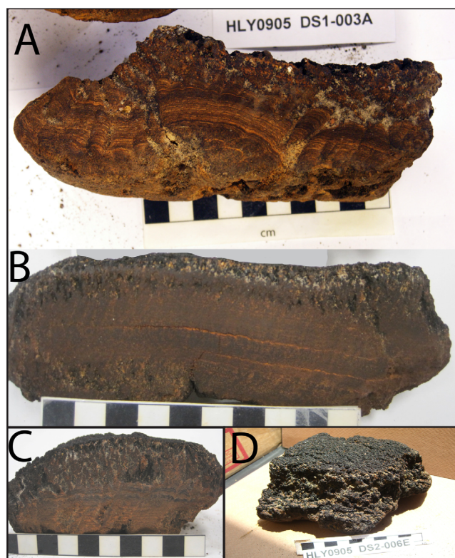
Figure 3. Photographs of cut surfaces showing stratigraphic layers in Fe-Mn crusts (a) HLY0905 DS1-003A, (b) HLY1202 DR2-001D, (c) HLY1202 DR5-D-D, and (d) uncut crust HLY0905 DS2-006E; note centimeter scale in each frame.
