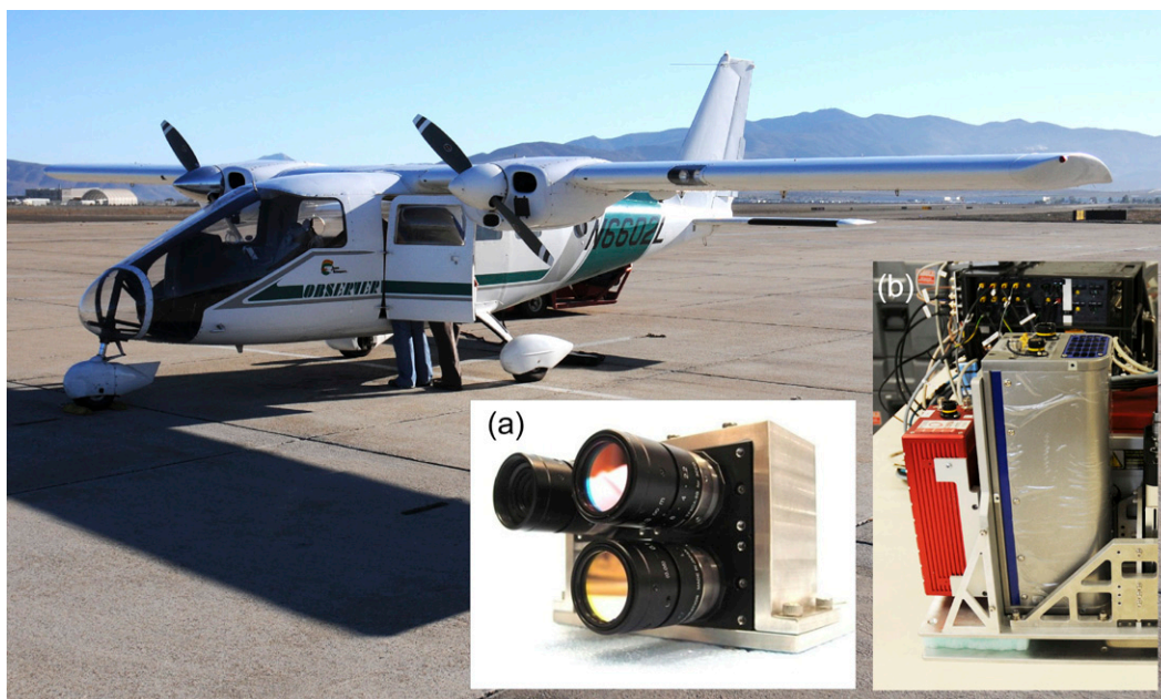
FIG. 2. Partenavia P68 Observer aircraft used during both experiments. (a) Multispectral dye fluorescence camera system used during IB09 and (b) hyperspectral pushbroom visible-to-NIR imager used during RIVET.
