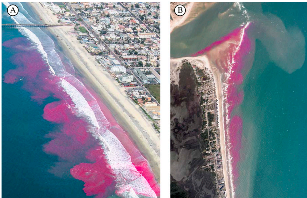
FIG. 1. Color-enhanced photographs of dye tracer released (a) within the surfzone at Imperial Beach, California, and (b) within an ebb tidal flow at New River Inlet, North Carolina. The structure of tracer ejected seaward of the surfzone is not resolved by sampling transects using jet ski and boat.
