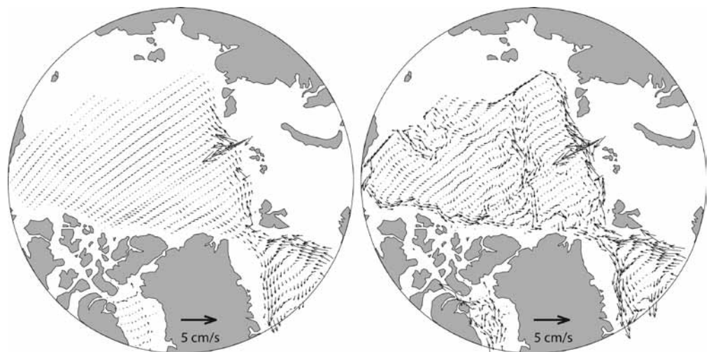
Figure 3. Time mean flow from Nucleus for European Modelling of the Ocean (NEMO) without the "neptune effect" (left) and with the neptune effect (right) at 551 m. The neptune effect (Holloway, 2009) is a theory that the many degrees of freedom expressed by ocean eddies will organize mean circulations. Neptune parameterization intensifies cyclonic (counterclockwise) boundary rim currents and better reproduces the circulation patterns shown in Figure 2. From Holloway and Wang (2009). Copyright 2009 American Geophysical Union. Reproduced by permission of American Geophysical Union
