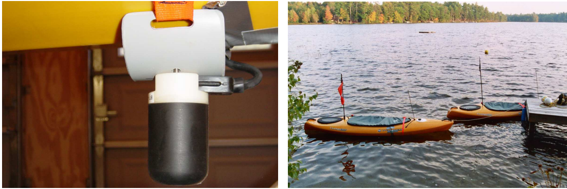
(a) Modem transducer strapped to the hull (b) Two kayakers moored on the pier while the a third one moves and determines its distance to the moored ones using the acoustic modem
