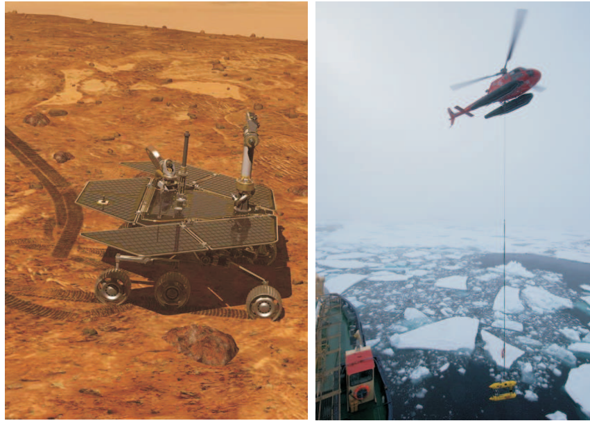
Figure 1-1: MER and Seabed , two exploration robots in a hostile environment. Left: Artist impression of MER on Mars. Courtesy NASA/JPL-Caltech. Right: Seabed deployed during the Gakkel Ridge Expedition in July 2008. Photo courtesy of Hanu Singh.
